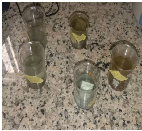
Figure 5. Mild steel and aluminium coupons immersed in 0.5M H_2SO_4 with unripe plantain peel and stem extract
