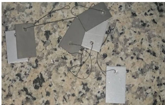
Figure 1. Threaded mild steel and aluminium coupons
