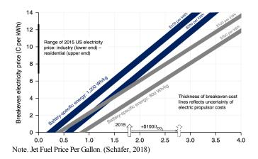
Figure 3. Break-even electricity price for a first-generation allelectric aircraft
