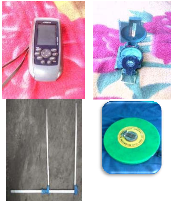
Figure 1. Material for taking impact data (GPS, Compass, Compact forestry and Double decameter)
